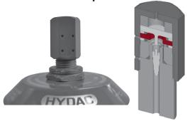
Protection by means of complete discharge in the case of excessive temperature and pressure.
