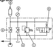
Note: When using hydro-pneumatic accumulators for stored hazardous energy, HYDAC recommends the use of its Safety and Shut-off Block (SAF) with solenoid operated bleed valve
