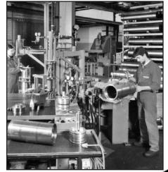
Assembly of Piston Accumulators
