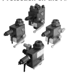
The fluid side has to be protected against excessive pressures with approved safety valves. HYDAC provides the pressure relief valve (*DB12 Series*) which has a pressure setting (*set by HYDAC*) up to 5800 psi (400 bar). The sealed valves carries a CE mark, and is integrated into the safety and shut-off blocks in nominal sizes DN10 to DN32.
