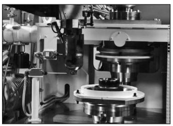
Electron-beam welding of diaphragm accumulators
