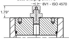
Gas Valve Version 1 (code designation VA) Uses Charging Unit FPK
