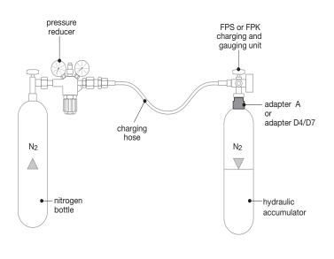
FPS Unit FPK Unit with Adapter D4/D7 with Adapter A\*
